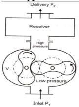
Lobe type air compressor: it is a rotary type of compressor consisting of two rotors which are driven externally.
