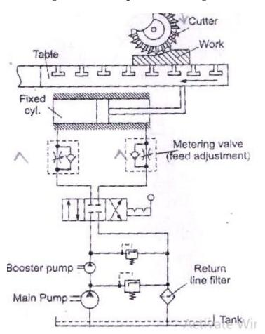
**Explanation:** - Hydraulic circuit for milling machine is comparatively different from other circuits. Table movement of milling machine is required to be adjustable for different feeds for different type of work. Therefore for both strokes of the cylinder, on both ends of cylinder flow control
