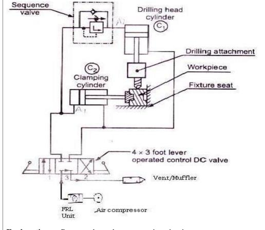
**Explanation:** Pressure dependent sequencing circuit:
