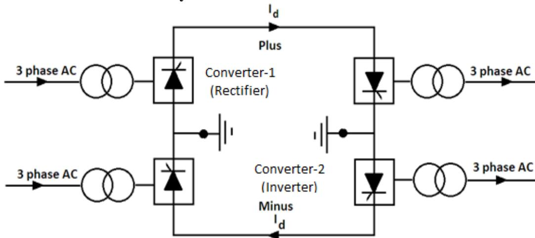
**Bipolar HVDC transmission system**
