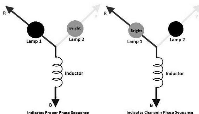
Connect two lamps, lamp1 to R-phase, lamp2 to Y-phase and inductor to B-phase as shown in the above figure. Resistors are connected in series with the lamps for protecting the lamps from over currents and breakdown voltages. If the sequence of supply is RYB, then the lamp 2 will glow brighter than lamp 1; if the sequence of the supply is reversed or altered, then the lamp 1 will glow brighter than the lamp
