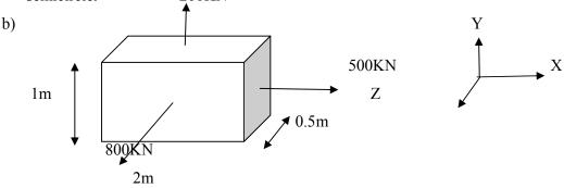
Find linear strains in x, y and z directions of the rectangular block loaded as shown in the figure. Hence using the linear strains values, find the total strain in z direction. Take E=200GPa. and Poisson's ratio=0.25
