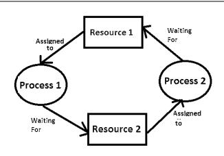
In this example, process 1 wants the resource 2 ex; scanner while holding the resource 1 ex: printer. Process 1 cannot proceed until both the printer and the scanner are in its possession.
