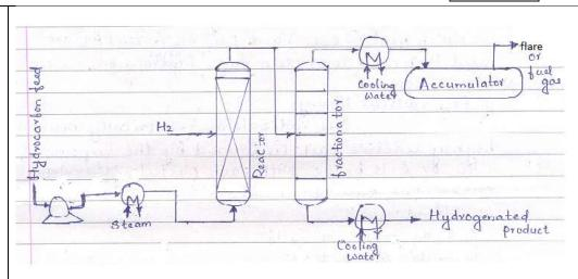
Hydrogen and hydrocarbon feed flows concurrently in a fixed bed reactor. Intimate mixing of hydrogen and reactants in the reactor bed is essential to make the best use of palladium catalyst. Poor hydrogen distribution results to inadequate diolefin hydrogenation. Additional equipment for high temperature hydrogen stripping is required for removal of polymer in order to extend the useful life of catalyst.
