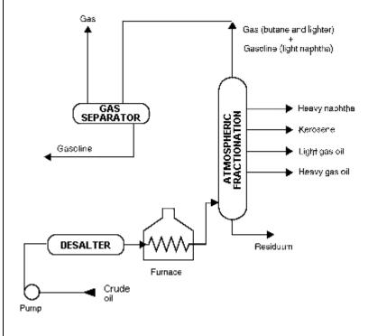
The crude oil is preheated to 350-380°C in tubular furnace known as pipe still.
