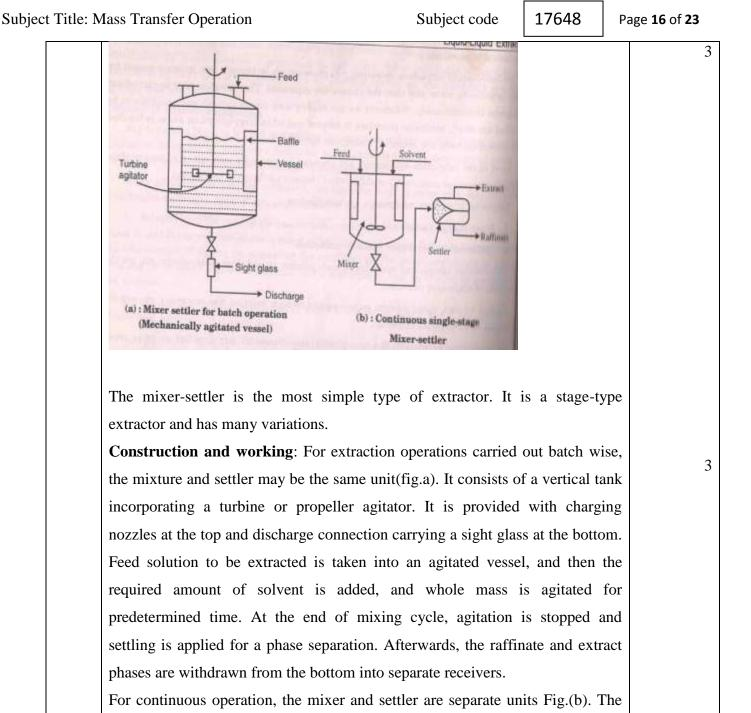
mixer is a small baffled agitated tank provided with inlet-outlet connections and settler is often a continuous gravity decanter. In this extractor, two phases are
