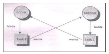
In this example, task #1 wants the scanner while holding the printer. Task #1 cannot proceed until both the printer and the scanner are in its possession. Task #2 wants the printer while holding the scanner. Task #2 cannot continue until it has the printer and scanner. Because neither task #1 nor task#2 is willing to give up what it already has, the two tasks are now deadlocked because neither can continue.
