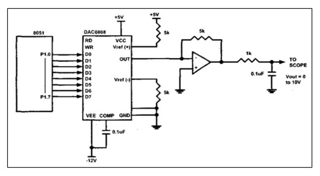
Assembly language program ORG 0000H MOV A, #00H :Load A=00H UP: MOV P1,A ;Send A to P1 INC Α ;Increment A NOP ;delay ;Compare A with Max. amplitude CJNE A, # 0FF, UP UP1: MOV P1,A ;Copy A to P1 DEC A ;Decrement A NOP ;delay CJNE A, #00H, UP1 ;Compare A with minimum 00H SJMP UP ;Repeat
