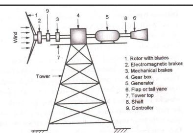
Fig- Horizontal axis wind turbine (02 marks for classification and 02 marks for figure )
