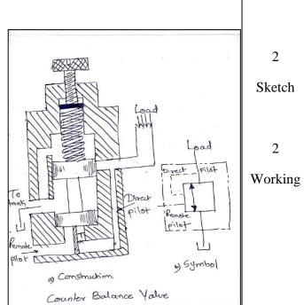
descending of the load. As this valve gets actuated line pressure, it is known as direct operated counterbalance valve.
