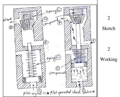
As and when we cut-off the pilot signal the flow from (A) and (B) will continue. When pilot signal will be cut-off, spring S1 and S2 will expand and moving poppet will again block the flow from (A) to (B).
