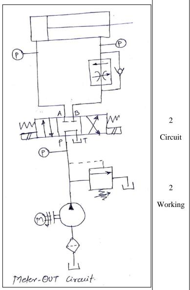
considered. With meter-out speed control, the quantity of oil leaving the cylinder is controlled. When the cylinder is extending, the oil from the rod-end is metered which a smaller quantity than that is flowing into the full bore end. Consequently, under extend conditions; meter-out flow control is not as sensitive as meter-in control. When the cylinder is retracting, the reverse is true.
