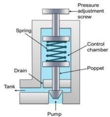
The pressure relief valves are used to protect the system components from excessive pressure. Its primary function is to limit the system pressure within a specified range. It is normally a closed type and it opens when the pressure exceeds a specified maximum value by diverting pump flow back to the tank.
