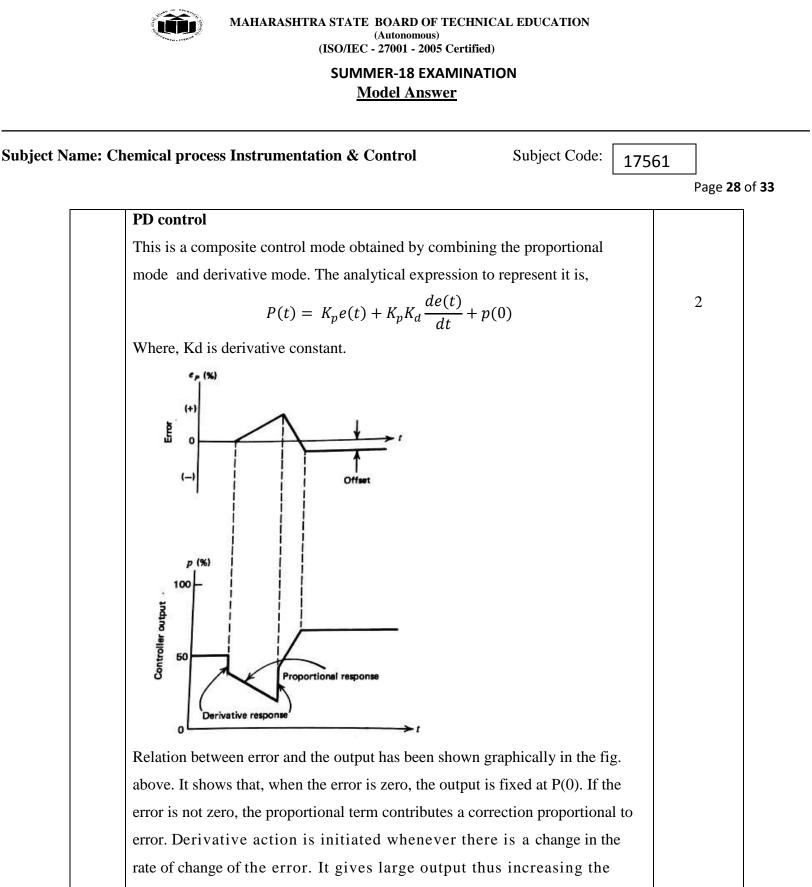
speed of the system. This cannot eliminate the off-set error, as the derivative
