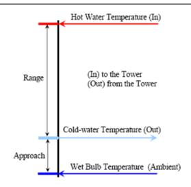
a) **Range**. This is the difference between the cooling tower water inlet and outlet temperature. A high CT Range means that the cooling tower has been able to reduce the water temperature effectively, and is thus performing well.
