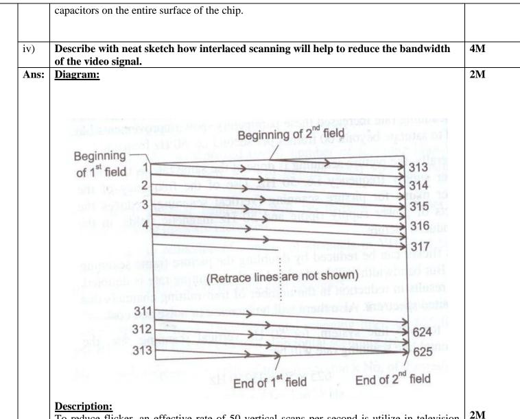
To reduce flicker, an effective rate of 50 vertical scans per second is utilize in television pictures system. This is accomplished by increasing the downward rate of travel of the scanning electron beam. By increasing downward scanning rate, every alternate line gets scan instead for every successive line. After the 1st scan the beam reach the bottom of picture frame, the beam quickly returns to the top to scan remaining lines which are missed in 1st scan.
