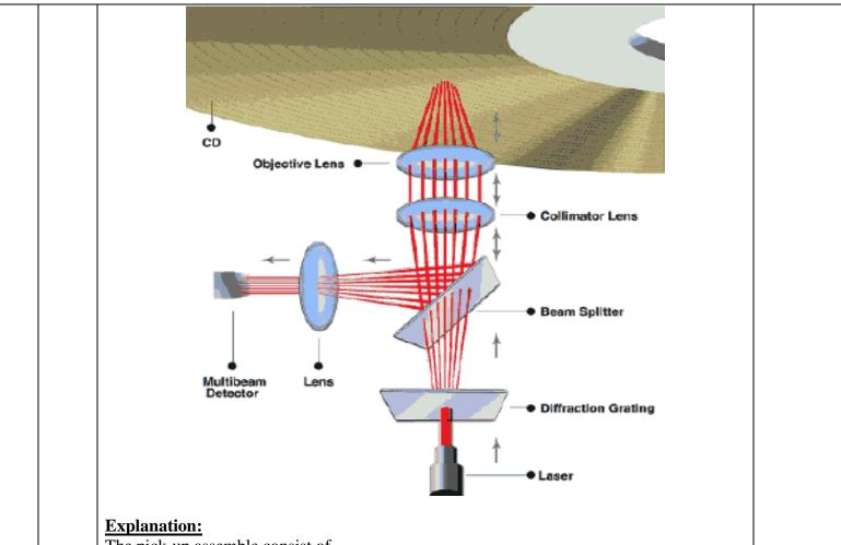
The pick-up assemble consist of –
