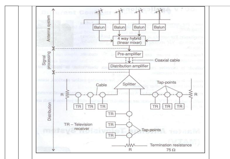
Master antenna TV system is used to deliver a strong signal (over 1mv). It is delivered from one or more antennas to every television receiver connected to the system. This type of system is implemented in the areas where signal strength is less. It is generally used in large hotels, motels schools and apartment building.
