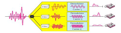
In FDM, signal generated by each sending device modulate different carrier frequencies. These modulated signals are combined into a single composite signal that can be transported by the link. Carrier frequencies are separated by guard bands to prevent over- lapping of signal. Though it is an analog multiplexing system, digital signals can also be sending by converting them into analog signals.
