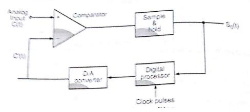
In this, the step size of the DAC is automatically varied depending on the amplitude characteristics of the analog input signal. When the output of the transmitter is a string of consecutive 1's or 0's, this indicates that the slope of analog signal either in +ve or -ve direction. The DAC has lost track of exactly where the analog samples are and the possibility of slope overload occurring is high. In ADM, the value of delta changes in accordance with the slope of the sampled analog input.
