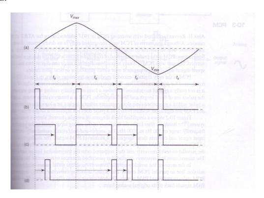
b) Define sampling theorem and draw waveform for natural sampling. (Theorem 2Marks, Relevant waveform 2Marks)
