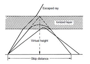
When the wave is refracted by the ionosphere it is bent down gradually rather than sharply. Below the ionized layer, the incident and refracted rays follow path that are
