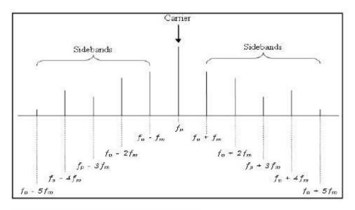
Figure 3. An FM signal's frequency spectrum
