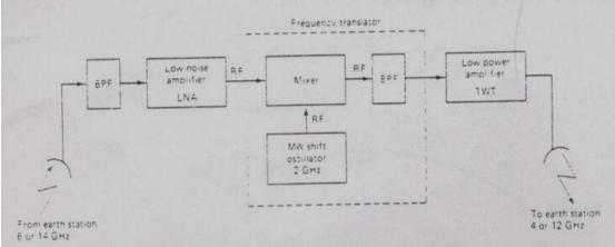
A typical satellite transponder consists of :
