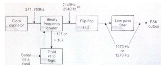
Note that binary 1 corresponds to frequency 1270 Hz and binary 0 to frequency 1070 Hz As shown in block diagram,
