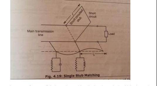
1. The most important feature of single stub matching is that the stub should be located as near to the load as possible.
