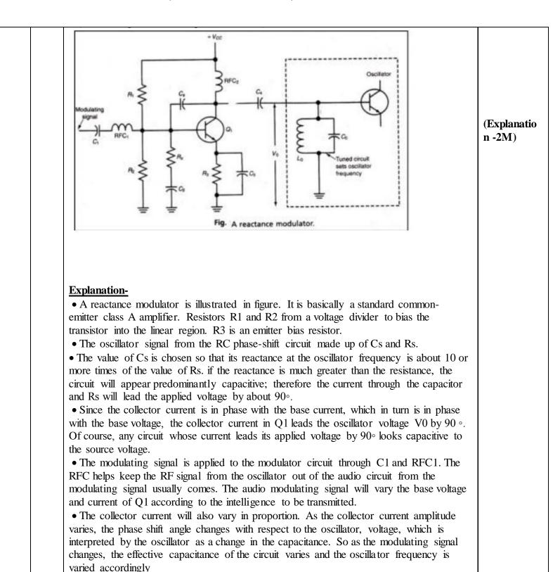
• An increase in capacitance lowers the frequency, whereas a lower capacitance increases the frequency. The circuit produces direct frequency modulations.
