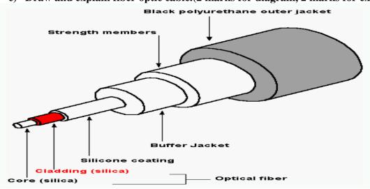
As shown in the figure, at the center is the glass core through which the light propagates. In multimode fibers, the core is typically 50 microns in diameter. In single mode fibers, the core is 8 to 10 microns. The core is surrounded by a glass cladding with a lower index of refraction than the core, to keep all the light in the core. A thin plastic jacket is used to protect the cladding. Fibers are grouped in bundles, protected by an outer sheath.
