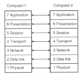
Fig: Horizontal Communication in OSI Model.
