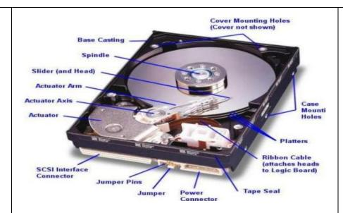
A hard disk drive is a sealed unit that a PC uses for nonvolatile data storage. Nonvolatile, or semi-permanent, storage means that the storage device retains the data even when no power is supplied to the computer.
