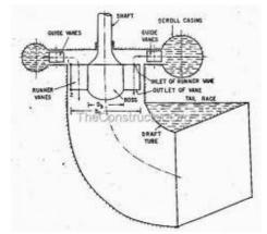
**Working:** it is a axial flow reaction turbine. It consists of main parts scroll casing, Guide vanes mechanism, hub with vanes or runner of the turbine and draft tube.
