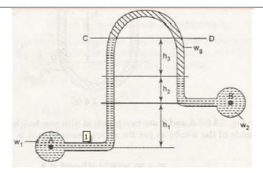
Pressure at C (left limb) = Pressure at D (right limb)
