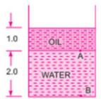
$= 9.8 \times 1000 = 800$  kg/m<sup>3</sup> pressure intensity at any point is given by
