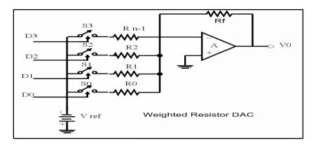
**Figure: Weighted Resistor DAC**
