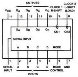
Figure: Pin diagram of IC 7495
