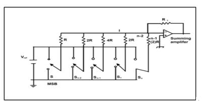
**Figure: Weighted Resistor DAC**
