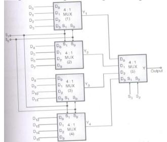
c) Design 16:1 multiplexer using 4:1 multiplexers only.(4 Marks)
