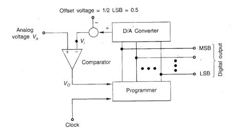
**Working:** The comparator serves the function of the scale, the output of which is used for setting/ resetting the bits at the output of the programmer. This output is converted into equivalent analog voltage from which offset is subtracted and then applied to the inverting input terminal of the comparator. The outputs of the programmer will change only when the clock pulse is present.
