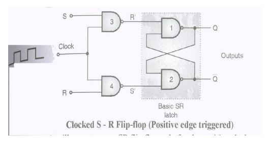
The positive edge triggered S-R flip Flop. It is also called as clocked SR FF. This circuit will operate as an SR flip flop only for the positive clock edge but there is no change in output id clock=0 or even for the negative going clock edge.
