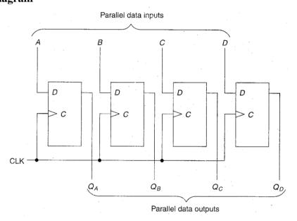
**Working:** In Parallel In-Parallel out Shift register, the data bits are entered simultaneously into their respective stages on parallel lines. The output data bits are also available on parallel lines. Immediately following the simultaneous entry of all data bits, the bits appear in the parallel outputs. **Truth Table**
