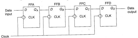
Working: This type of register accepts data serially i.e. one bit at a time on a single line. It produces the stored information on its output in serial form.
