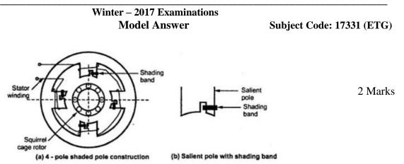
It has squirrel cage rotor and salient pole stator. The stator poles are shaded partially by short circuited conductor band to create the phase difference between the fluxes emerging from shaded and un-shaded portion. These phase differing fluxes produce the required torque on the rotor for motion.
