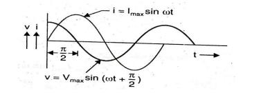
iv) Waveform of voltage and current for ac circuits containing Capacitance and resistance:
