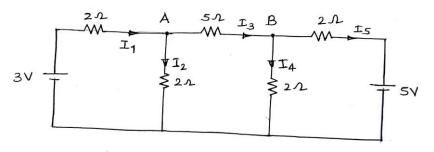
At node A  $I_2 + I_3 = I_1$   $\frac{V_A}{2} + \frac{V_A - V_B}{5} = \frac{3 - V_A}{2}$ Multiplying by 10 to both sides  $\left(\frac{V_A}{2} \times 10\right) + \left(\frac{V_A - V_B}{5}\right) \times 10 = \left(\frac{3 - V_A}{2}\right) \times 10$
