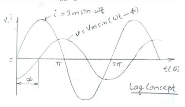
Lagging Phasor Representation: Voltage (V) lagging current (I) by angle  $\Phi$
