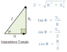
e) A choke coil is connected across 230 V, 50 Hz supply. The power consumed by the coil is 960 W and current is 8amp. Calculate circuit constants (R and L). Given:
