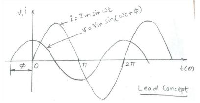
Leading Phasor Representation: Voltage (V) leading current (I) by angle  $\Phi$
