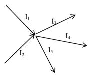
In the above example,  $I_1 + I_2 = I_3 + I_4 + I_5$
