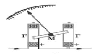
Where F = Fixed Coil; M – Moving Coil
