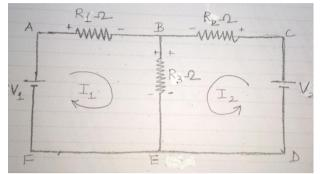
Applying KVL to Loop ABEFA,  $V_1$ -  $I_1R_1$ -  $(I_1+I_2)R_3 = 0$ Applying KVL to Loop BCDEB,  $V_2$ -  $I_2R_1$ -  $(I_1+I_2)R_3 = 0$ (Potential rise considered to be positive and potential drop to be negative)
