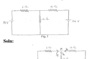
Applying KCL at Node A,  $i_1+i_{3=i_2}$
