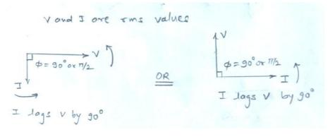
ii) Voltage equation and current equation  $v = V_m \sin wt$  (1/2 Mark)
