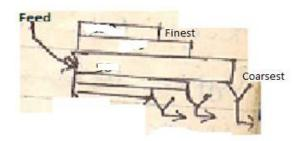
The innermost one is the longest and has coarsest perforations. The outer ones are successively shorter and have finer perforations.
