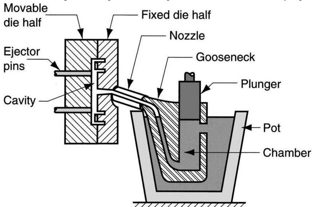
**Figure: Hot chamber die casting**
