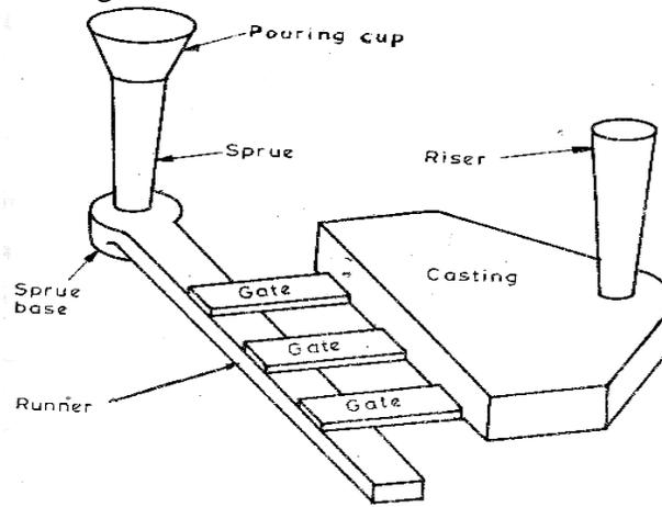
Figure: Gating system in casting.
