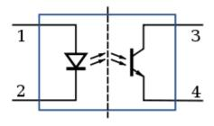
**Usage**: opto-isolator contains a source (emitter) of light, almost always a near infrared light-emitting diode (LED), that converts electrical input signal into light, a photosensor, which detects incoming light and either generates electric energy directly, or modulates electric current flowing from an external power
