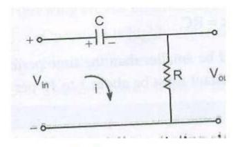
Fig: RC differentiating circuit
