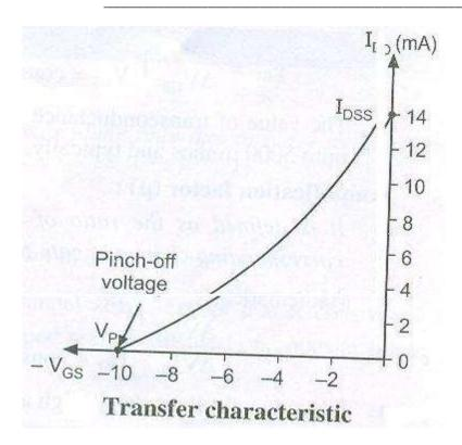
$I_{dss}(Shorted\ Gate\ Drain\ Current):\ It\ is\ the\ drain\ current\ with\ source\ shorted\ to\ gate, i.e.\ Vgs=0\ and\ drain\ voltage\ is\ equal\ to\ pinch\ off\ voltage.$
