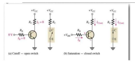
When the input voltage is positive both BE and CB junction are forward bias, therefore transistor is ON. Current $I_c$  increases and the output voltage decreases.
