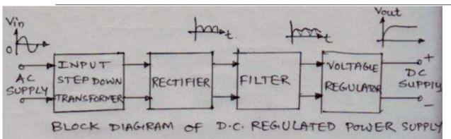
Explanation-Transformer- Step downs the 230 v AC into low voltage AC Vm Rectifier- Converts AC into DC.
