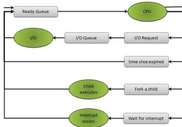
The above figure shows the queuing diagram of process scheduling.
