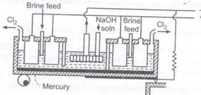
The cell contains a large angular trough with a layer of mercury at the bottom and divided into two compartments in the SLATE PARTITION not touching the bottom. Thus Hg in one compartment can flow into the other but any solution in one compartment cannot flow into other. The left hand compartment is fitted with graphite anode dipping in brine whereas the right hand compartment is fitted with iron cathodes dipping in dilute NaOH solution.
