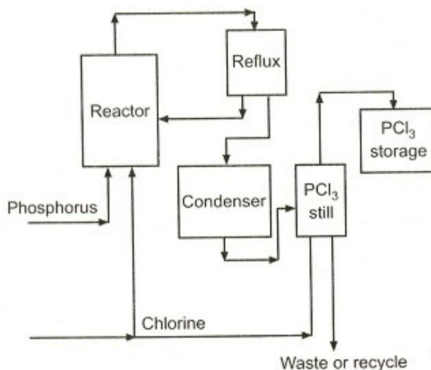
Liquid phosphorous and chlorine gas are fed in reactor.  $PCl_3$  formed is partly refluxed in the reflux and a part is passed through a condenser and then to a still for distillation and finally for storage.
