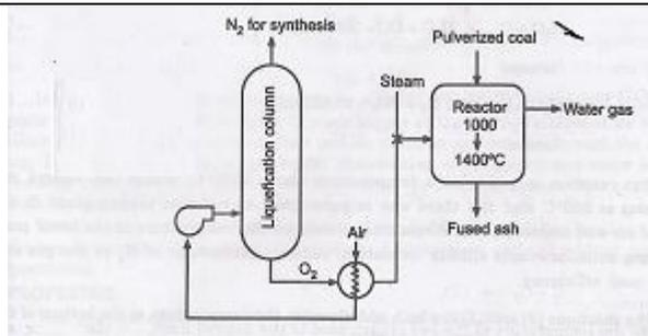
Process Description- Nitrogen is separated from air by liquefaction process.
